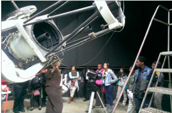
In order to keep their view sharp, the telescope mirrors must be periodically cleaned and given new silver reflective coatings. Since the primary mirror weighs 140 pounds and is built into the telescope support structure, this requires unscrewing 80 bolts that hold the telescope together.
