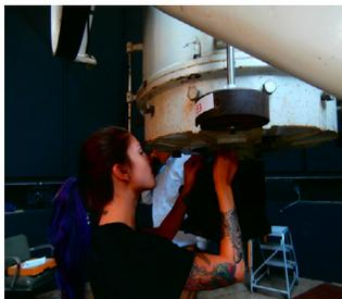
They then lifted out the mirrors, winched them down the observatory staircase, and sent them off to a professional cleaning facility. While the mirrors were out of the way, the telescope structure was repainted. A few months later, the mirrors came back and the disassembling procedure was reversed. The telescope now
