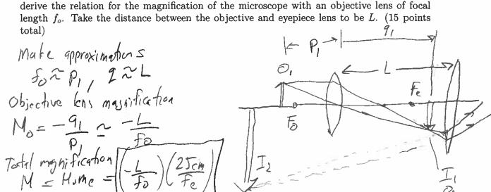
**Problem 4.** Starting with the magnification relation for the eyepiece  $m_e = (25 \text{ cm})/f_e$ ,
