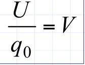
Where V is the <u>electric potential</u> with units of 1 J/1 C = 1 volt or 1 V
